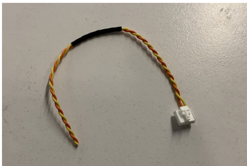
Figure 3, Door Station and Card Reader, Security Module Cable (101512130 RS-485, PHS4 to 2OPEN, 150 mm, yellow/orange)
