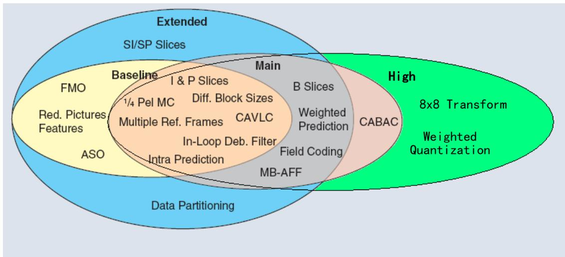
Figure 1 H.264/AVC Profiles and Encoding Technology Tools
